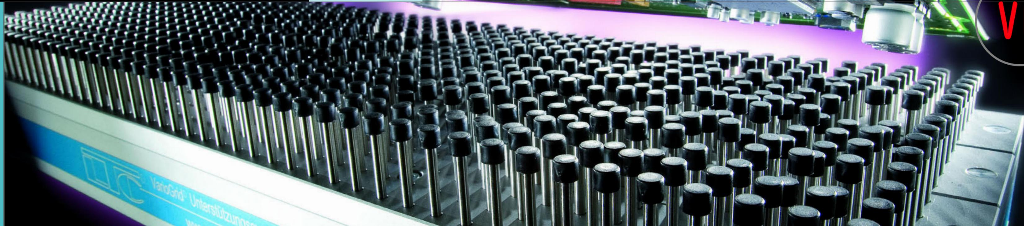
The installation and operation of the VarioGrid® system is as easy as 1-2-3. Just position the VarioGrid® system modules within the working area, place the control unit near the interface of the system and connect the pneumatic tubing according to the installation instructions.
